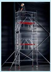
The Eiger 500 AGR Ladder Span is an alternative to the standard tower, with fewer components for a quick easy build method. The guard rail is positioned before the operator ascends the platform to ensure a safe system of work. A very rigid tower with easy to use AGR frames.
