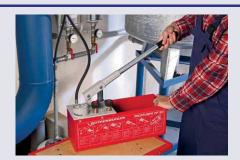
Pressure testing pump for conducting hydrostatic pressure tests on water or oil carrying pipework systems and vessels.
