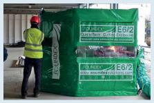
This extremely robust 2.5m2 industrial quality cutting enclosure incorporates acoustic walls and roof with quick access entrance and left and right ports to accommodate extra long lengths of material.
