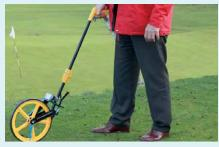
This is widely used for road and ground measuring and is ideal for measuring long distances where a long tape becomes impractical.
