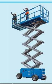
A diesel powered rough terrain 4 wheel drive machine with slide out platform extension decks for added workspace.
