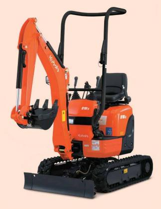
Ideally suited for working in back gardens or other areas with very limited access this machine will pass through a standard 760mm gate or doorway. It's expanding track system gives additional stability when working and the roll bar can be folded down to allow access through low level areas. User-friendly controls allow this machine to be used for a wide range of landscaping and other small projects.
