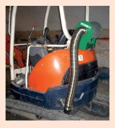
This is generally used when diesel engines are run within an enclosed environment and therefore ventilation is restricted. The Ravex range of exhaust filters are specifically designed for use on diesel powered plant and construction equipment to effectively reduce smoke and particulate emissions from engines.
