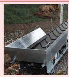
Robust Portable conveyor able to be linked, Ideal for moving soil and debris out of basements, across lawns etc.
