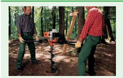
A robust two man auger for drilling post holes.
