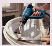
Heavy duty hot air stripper with a variable temperature control. An ideal tool for stripping
