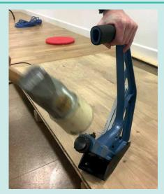
A fast and effective way to lay traditional tongue and groove floorboards, simply position the tool and strike plunger with mallet supplied.
