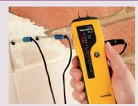
Pin type moisture meter, compact design for assessing levels of moisture in building materials such as wood, masonry, drywall, plaster and
