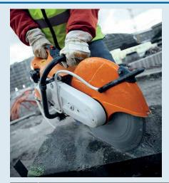
The construction industry workhorse, this 2 stroke petrol machine will cut most materials to a maximum cutting depth of 100mm (300mm version) or 125mm (350mm version). Diamond or abrasive blades are charged in addition to the hire of the machine.
