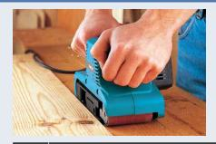
To smooth rough, flat timber surfaces quickly and effectively.
