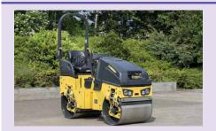
These are Ideal for compacting large areas of stone, hardcore or asphalt. The Ride on Rollers have a compaction force of 1040kg and due to easy manoeuvrability, they provide excellent results.
