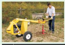
The hydraulically driven hole borer is a one-man operation with a choice of augers. It can drill a hole up to 96cm deep.
