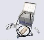
The best way to carry out essential pipe work or maintenance without draining down the entire system. Two ice plugs are created allowing the pipe to be cut. Ideal for copper, iron, lead or plastic cold water pipes from 8-42mm diameter.
