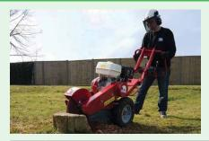
The tough tungsten tipped blade will make quick work of most tree stumps. This carefully balanced tool reduces unwanted stumps to fine chippings, cutting down below the surface.
