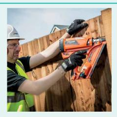
The IM350+ Cordless 1st Fix Framing Nailer powered by a fuel cell and a rechargeable li-ion battery. Ideal for framing applications such as stud work, noggins, roof battens and fencing. Drives 51-90mm pails.
