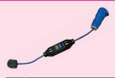
Safety device that monitors electrical flow to a tool and instantly cuts power if any change occurs, reducing the risk of injury by electric shock. Essential when working with power tools from a 240V supply.
