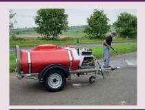
A road towable 940ltr Diesel Powerwasher. This highly versatile unit allows for cleaning or drain maintenance to be carried out in even the most remote locations where the water supply is restricted.
