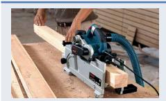
Ideal for planing to size and for producing the highest surface quality finish. The 82mm base will remove over 2mm in a single pass.
