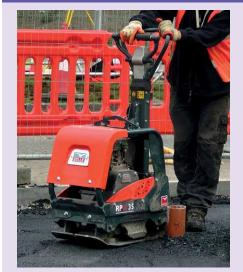
Heavy duty reversible plate compactor with hydraulic shift gearbox for changing movement
