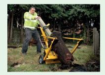
The Post Puller removes fence posts, gate posts, bollards and street furniture.
