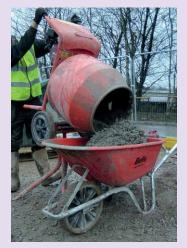
Available in 110V & 240V electric, or in petrol versions, these lightweight compact mixers come with a rotating stand for tipping into wheelbarrows.
