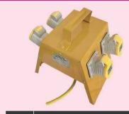
This 110V Junction box, also known as splitter box or spider is perfect for use on site for connecting multiple power tools up to a single transformer. Checks should be made prior to use to establish that the power supply can handle an increased load.
