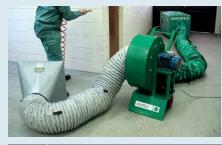
The VENTEX 300SCF Centrifugal Fan is particularly suited to extracting any hot fumes or paint fumes because the motor is not in the airflow, also where long duct runs are required to remove the fumes to atmosphere.
