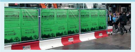
The Contractor curtain and quilt are excellent for general noise control with a BS EN rated attenuation of 28.2dB. The quilt size corresponds to a 3.5m temporary fence panel, for convenient installation. Patented Velcro side connection enables a seamless noise barrier of greater integrity, and eyelets enable suspension from site fencing, scaffolding and hoardings.
